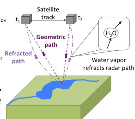
**Fig. 1. Water vapor delays radar path.**
